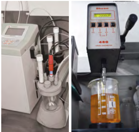
Titration of chemical compounds. Determination of viscosity.
