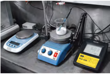
PH metric titration of resin powder.
