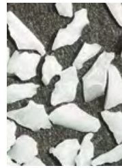
Ceramic grains viewed under a microscope.
