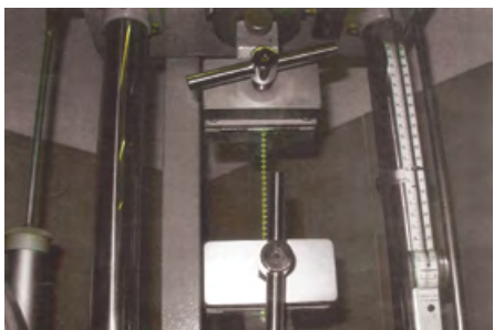
Yarn resistance test of fiberglass reinforcements.
