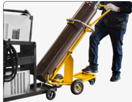
LOAD ONTO CART
