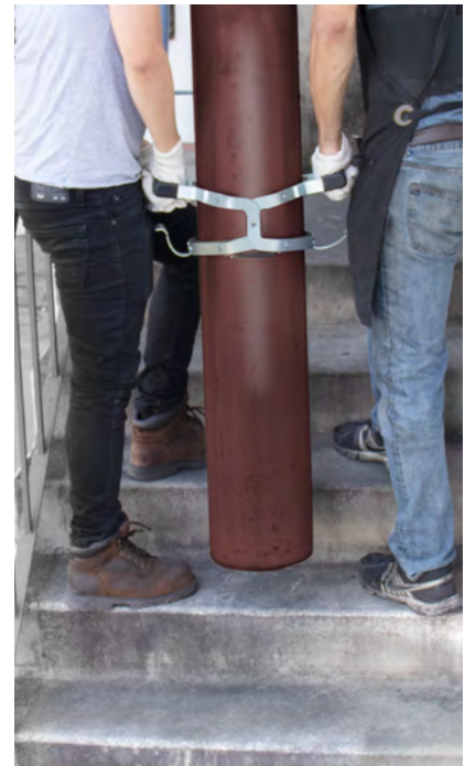
Safely carry heavy cylinders upstairs with the Gas Grabber.
