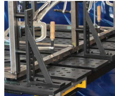
Insert V-Blocks to support round stock.
