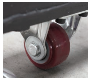
Two casters for quick repositioning of manipulator.
