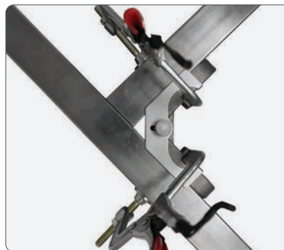
Retractable Plate Makes edge alignment a snap.
