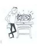
**16.** Disconnect tools before servicing and when changing accessories such as grinding wheels, polishing mops, grinding belts, blades, bits, cutters, etc.
