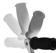
The rocking handle of the power tool can be secured in five different positions. Using different angles of the forward hand grip eases work load in different working positions. For right- and left-handed users. To tilt the handle, unscrew the handle for a few turns, bring the handle in the desired position, lock the handle by screwing it snug.
